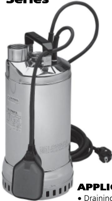
Submersible pumps for clean and slightly dirty water manufactured in AISI 304 stainless steel. Head up to 20 metres, delivery up to 420 l/min (25,2 m<sup>3</sup>/h). Four basic models with 0,55 to 1,5 kW.
